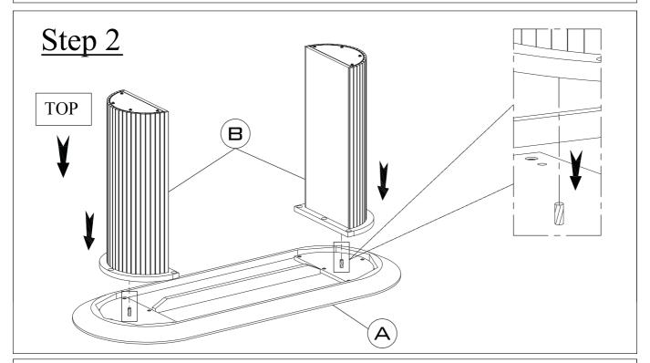
Using a second person to assist you, position the Leg Frame (B) upside down, and align the corresponding hole with the previously installed Dowel (H-1). Lower the Leg Frame (B) onto the Table Top (A) and align the through holes in the Leg Frame (B) with the threaded inserts in the Table Top (A).
