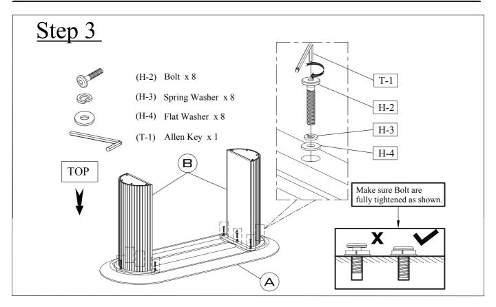
Secure the Leg Frames (B) to the Table Top (A) by first engaging all Allen Bolts (H-2), Spring Washers (H-3), and Flat Washers (H-4), stacking the hardware in the order as shown. Once all are engaged, fully tighten using the provided Allen Key (T-1). Do not over tighten.
