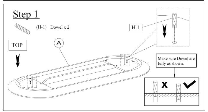
Using a second person to assist you, carefully place the Table Top (A) upside down onto a padded, non-marring surface. Insert Dowels (H-1) into the center of each circular support on the bottom of the Table Top (A).
